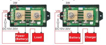
The figure above applies to batteries or circuits where the VAT1200 measures 0-100V; at this time, note that the jumper cap must be connected to 3W and need to use DC 10-30V power supply. The DC voltage supplies power to the measurement module; the wiring method on the left is suitable for the discharge measurement of the battery and the measurement of the DC circuit; the wiring method on the right is only suitable for the charge measurement of the battery.
