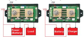
The above figure applies to VAT1200 measurement circuit voltage of 10-100V; please note that the jumper cap connected to 2W at this time, the left wiring method is suitable for battery discharge measurement and DC circuit measurement; The wiring method on the right is only suitable for battery charge measurement.
