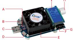
A. External wiring port, can be used by welding terminals
