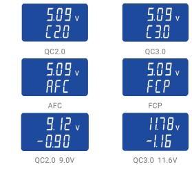
Upper line display the real-time voltage Bottom line display the voltage of selection
