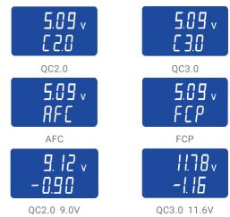
Upper line display the real-time voltage Bottom line display the voltage of selection
