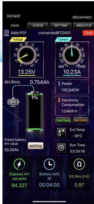
Figure 3-5-55 Over-voltage protection status
