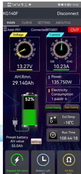
Figure 3-5-12 Over-voltage protection status
