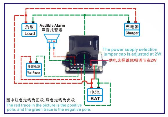
Note: The working power of the sound alarm is provided by an external power supply. If the sound alarm is used, an external power supply with the same working voltage as the sound alarm must be provided. Connect the positive and negative terminals of the sound alarm to the (+RELAY-) controller interface.
