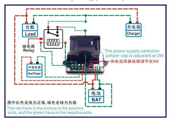
Note: The working power of the relay is provided by an external power supply. If the relay is connected, an external power supply with the same working voltage as the relay must be provided. Connect the control port of the relay to the (+RELAY-) controller interface.
